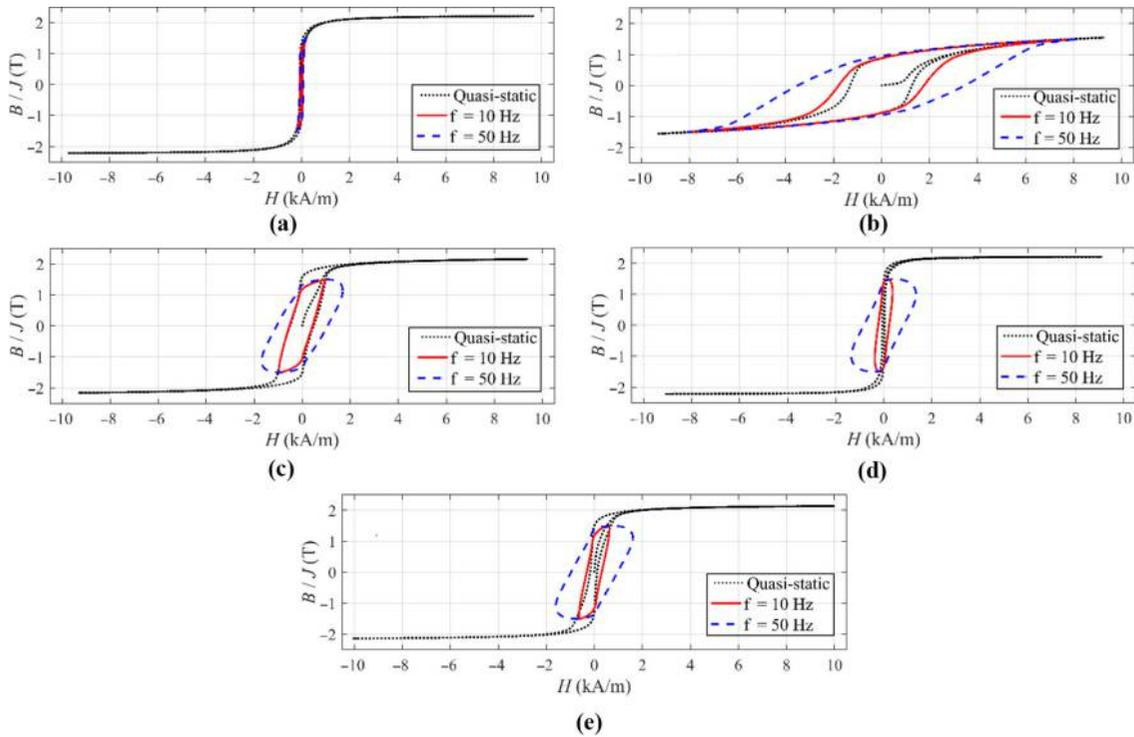
**Notes:** (a) Fe-Co-V laminated, HT1; (b) Fe-Co-V, as-built; (c) Fe-Co-V, HT1; (d) Fe-Co-V, HT2; (e) Fe-Co-V, HT3
