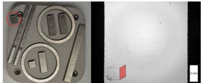
Note: A sample used for porosity analysis is marked with a red circle
