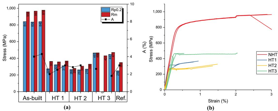
**Notes:** (a) 0.2 yield strength (Rp0.2), tensile strength (Rm) and elongation after fracture (A); (b) stress-strain curves (NHT = As-built)
