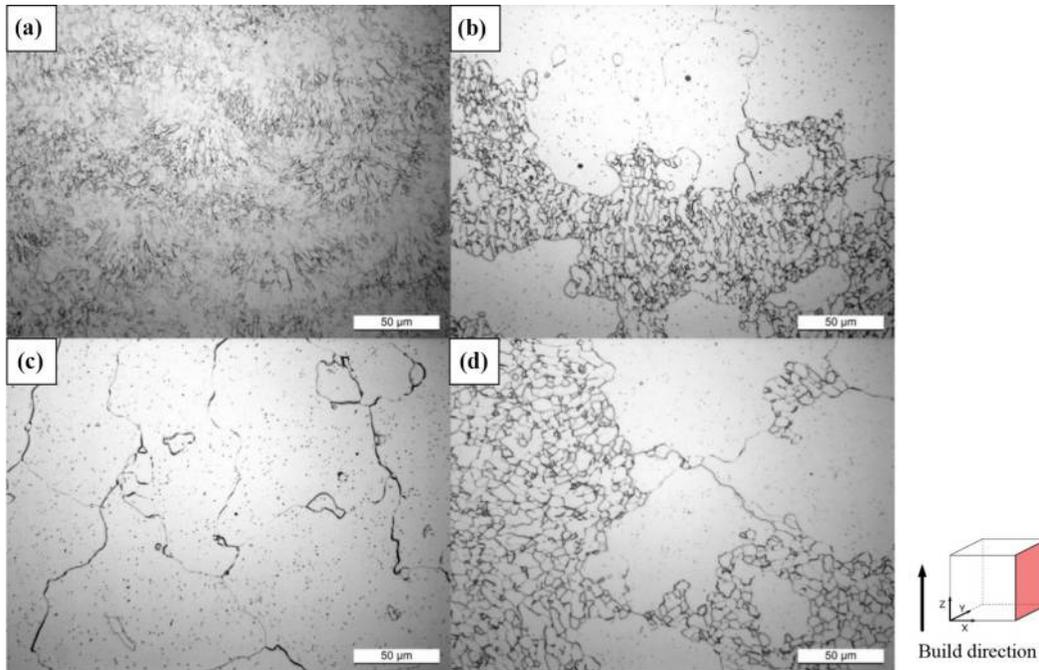
**Notes:** (a) As-built; (b) HT1; (c) HT2; (d) HT3**Figure 4** SEM images of 3d printed Fe-Co-V samples showing the solidified structure in the as-built sample (left) and the grain boundary precipitates in the heat treated sample containing Niobium
