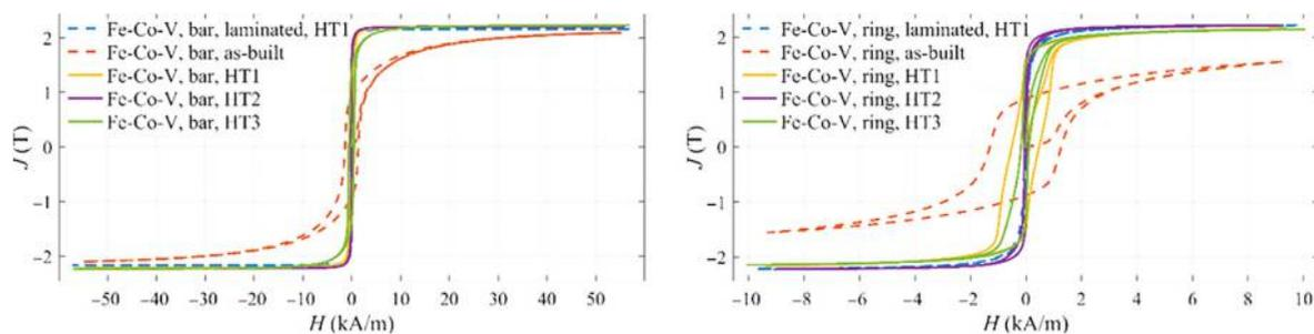
Notes: Left: Quasi-static measurement of bars up to 50 kA/m. Right: Quasi-static measurement of rings up to 10 kA/m
