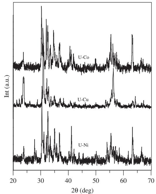
Fig. 1. XRD patterns of the  $Ba_4X_2Fe_{36}O_{60}$  ( $X = Co, Ni$  and  $Cu$ ) hexaferrites sintered at  $1275^\circ C$  for 6 h.
