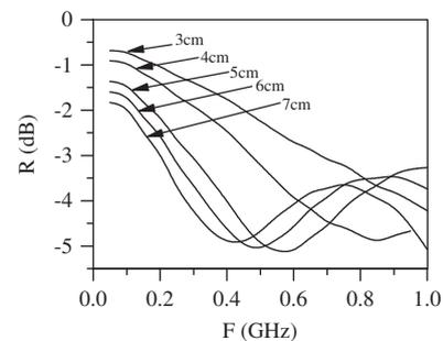
Fig. 10. Reflection loss spectra for the  $\text{Ba}_4\text{Cu}_2\text{Fe}_{36}\text{O}_{60}$  based composites.
