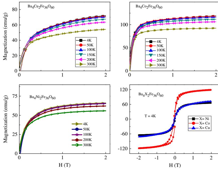
Fig. 2. Field dependent magnetization for the  $Ba_4X_2Fe_{36}O_{60}$  ( $X = Co, Ni$  and  $Cu$ ) hexaferrites measured at selected temperatures.
