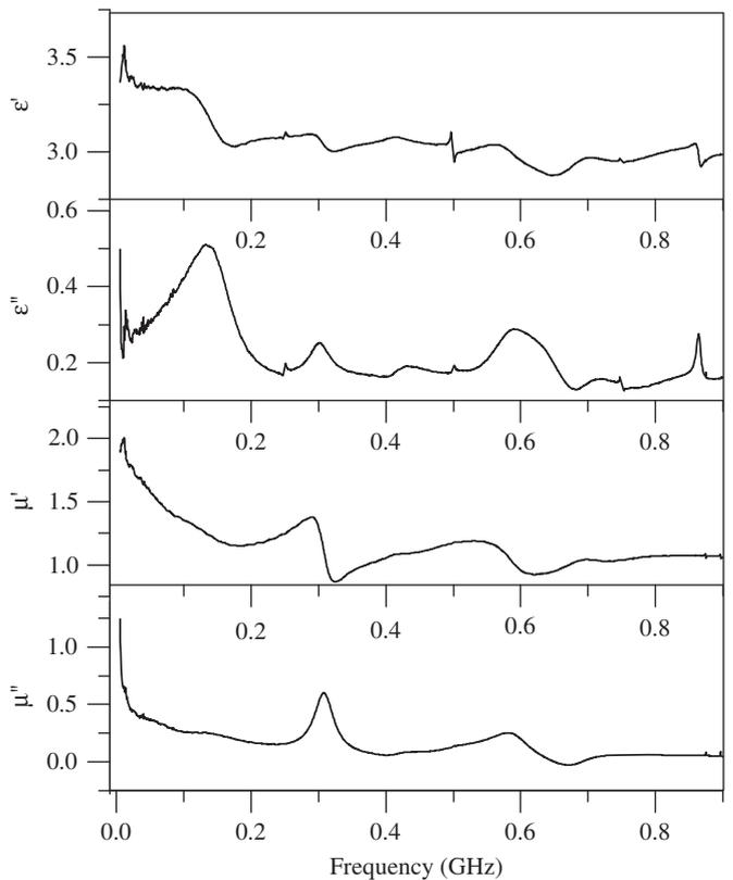
Fig. 6. Frequency variation of dielectric permittivity and magnetic permeability spectra of the  $\text{Ba}_4\text{Ni}_2\text{Fe}_{36}\text{O}_{60}$  based composites.
