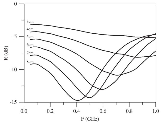
Fig. 9. Reflection loss spectra for the  $\text{Ba}_4\text{Ni}_2\text{Fe}_{36}\text{O}_{60}$  based composites.
