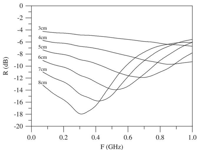
Fig. 8. Reflection loss spectra for the  $\text{Ba}_4\text{Co}_2\text{Fe}_{36}\text{O}_{60}$  based composites.
