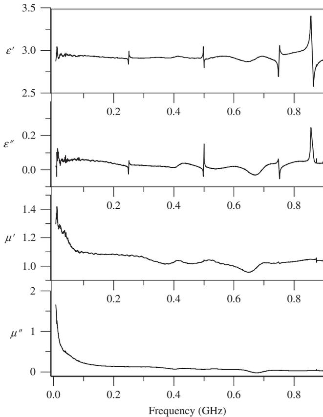
Fig. 7. Frequency variation of dielectric permittivity and magnetic permeability spectra of the  $\text{Ba}_4\text{Cu}_2\text{Fe}_{36}\text{O}_{60}$  based composites.
