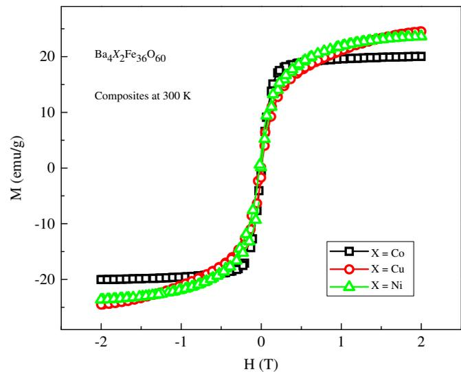
Fig. 4. Field dependent magnetization for composites of the  $\text{Ba}_4\text{X}_2\text{Fe}_{36}\text{O}_{60}$  ( $X = \text{Co}, \text{Ni}$  and  $\text{Cu}$ ) measured at 300 K.
