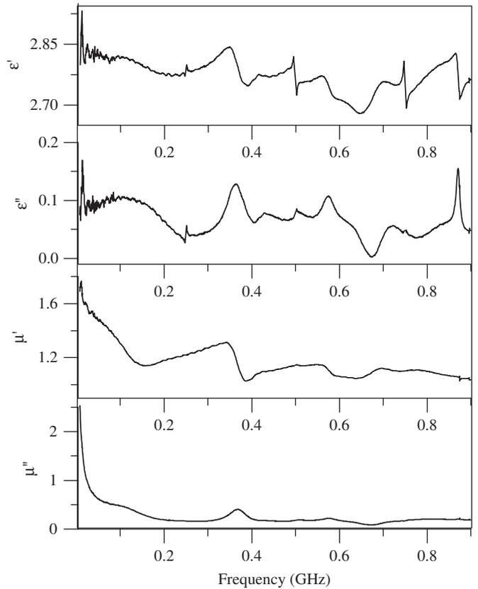
Fig. 5. Frequency variation of dielectric permittivity and magnetic permeability spectra of the  $\text{Ba}_4\text{Co}_2\text{Fe}_{36}\text{O}_{60}$  based composites.
