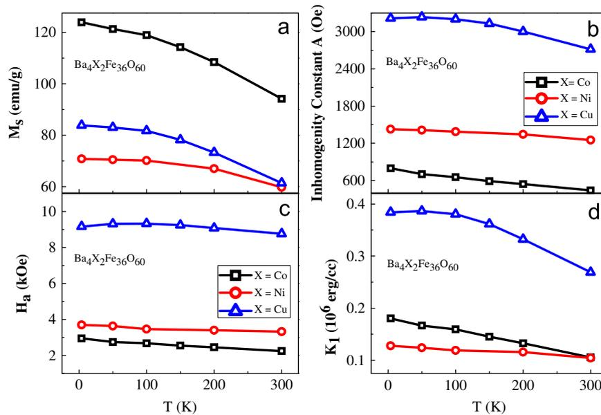
Fig. 3. Temperature dependence of (a) saturation magnetization ( $M_s$ ), (b) inhomogeneity constant ( $A$ ), (c) magnetocrystalline anisotropy field ( $H_a$ ) and (d) magnetocrystalline anisotropy constant ( $K_1$ ) for the  $Ba_4X_2Fe_{36}O_{60}$  ( $X = Co, Ni$  and  $Cu$ ) hexaferrites.
